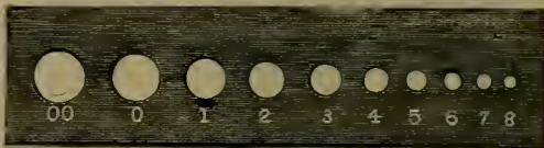
Sizes of Rivet Set Holes.
